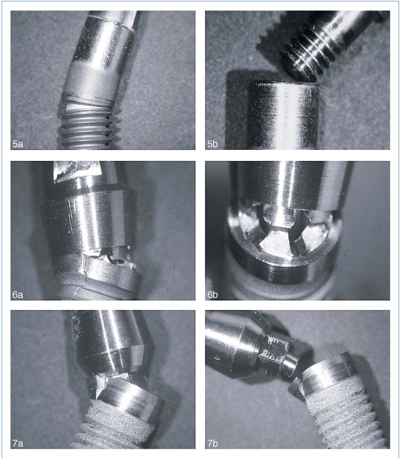
FIGURES 5-7. FIGURE 5. (a and b) Examples of failure mode for Unipost. FIGURE 6. (a and b) Examples of failure mode for Spline. FIGURE 7. (a and b) Examples of failure mode for Screw-Vent.
