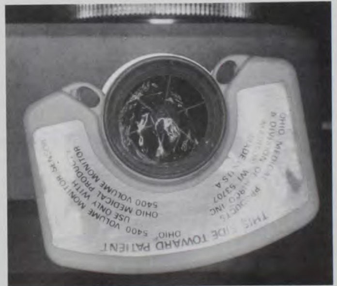
FIG. 1. Plastic disc abutting upon volume monitor sensor in expiratory limb.
