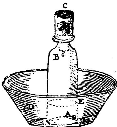
FIG. 1. Scheele's experiment (before 1775). Bees, honey and oxygen in the glass vessel, inverted in lime water.
