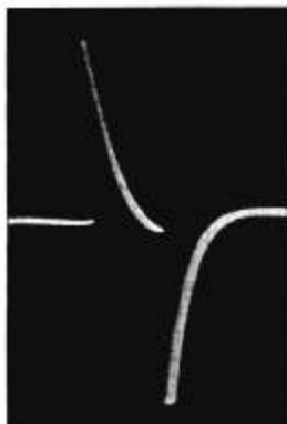
FIG. 1. Single electrical impulse used by catheter localizer.
