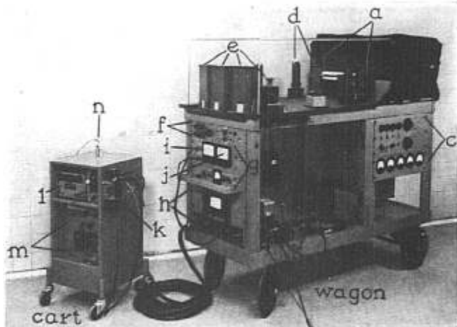
FIG. 3. Apparatus assembled for clinical study: a . Camera. b . Light-tight film box. c . Light control panel. d . Light sources. e . Heiland and Rubicon galvanometers. f . Main control panel. g . Acoustic gas analyzer. h . Cardiotachometer. i . Base gas meter. j . Ether meter. k . Telephones. l . Beckman oxygen meter. m . Panel with gas channel control valves, manometers and ether absorber. n . Oximeter earpiece.
