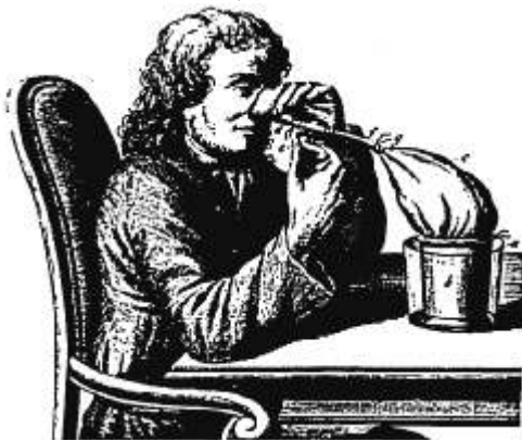
FIG. 1. Ingen Housz method of breathing oxygen and purifying the air of carbon dioxide used in 1781. The cylinder contained water but preferably limewater—"And in this way one can again free the dephlogisticated air after each breath of its aerial acid, for which use limewater is preferable to rain water." Reported in the Proceedings of the Batavian Society of Experimental Philosophy at Rotterdam (42). (Illustration taken from Ingen Housz' original work.)
