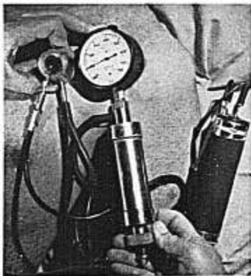
FIG. 1. Modification of Scarborough's petechiometer showing light with remote battery case, and syringe type vacuum pump.
