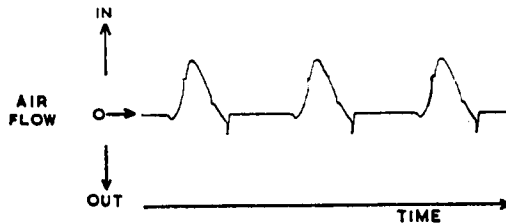
Pneumotachogram of inflow into Palmer-Starling 'ideal' pump.
