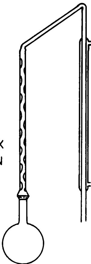
FIG. 1. Vigreux distilling column: distilling flask 50 ml. capacity, S. T. 14/20; Vigreux column 30 cm.; water jacket of condenser 20 cm. Ball and socket joint employed between Vigreux column and condenser for greater mobility.
