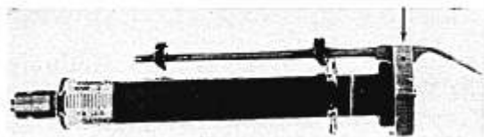
FIG. 1. Attachment to syringe for equilibrating fixed quantities of blood and air. The rod carrying the stops is hinged at the arrow.
