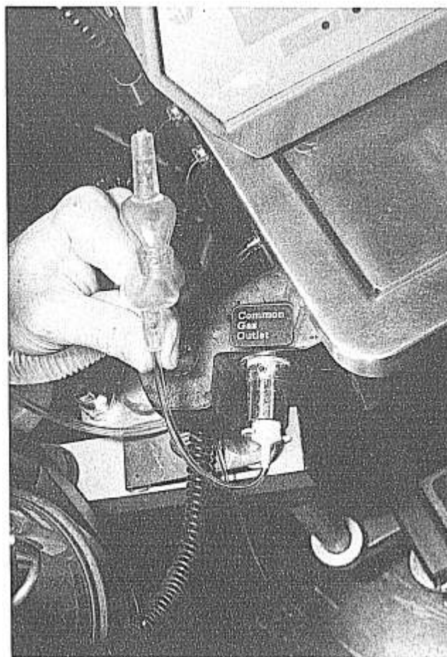
Fig. 1. An inverted pump from a Y-type blood set attached to a 2.5-mm inner diameter endotracheal tube adapter applies sustained suction to identify leaks in the low-pressure system even if a check valve is present in the common gas outlet.
