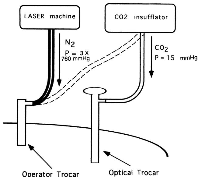
**Fig. 1.** Schematic representation of the laser machine showing the misconnection between the line delivering  $N_2$  and the operator trocar. The adequate connection that should have been used is represented by the dotted line. When the laser fired,  $N_2$  was insufflated into the peritoneal cavity at a pressure of  $3 \times 760$  mmHg.
