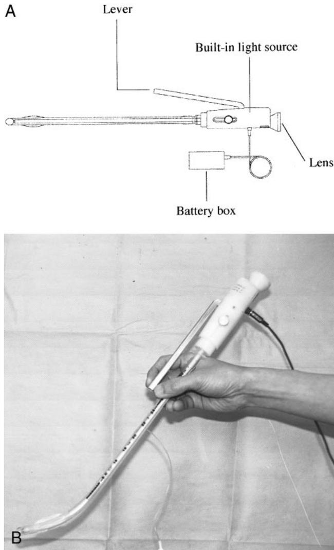
**Fig. 1.** The new fiberoptic stylet scope (FSS), StyletScope. (A) Diagram of the new FSS. By depressing the lever of the proximal handle, the distal tip of the stylet, together with the endotracheal tube, can be flexed 75° (B).
