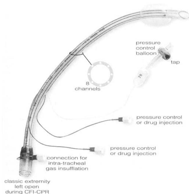
**Fig. 1.** Schema of the Boussignac-type multichannel endotracheal tube with the eight capillaries inserted in the wall of the tube. Note that the external extremity is left open to atmosphere during continuous insufflation of oxygen and cardiac massage.
