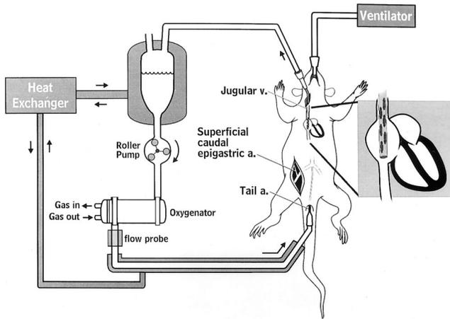
Fig. 1. Schematic diagram of the surgical preparation and rat cardiopulmonary bypass apparatus. Modified from Grocott *et al.*<sup>21</sup> with permission.
