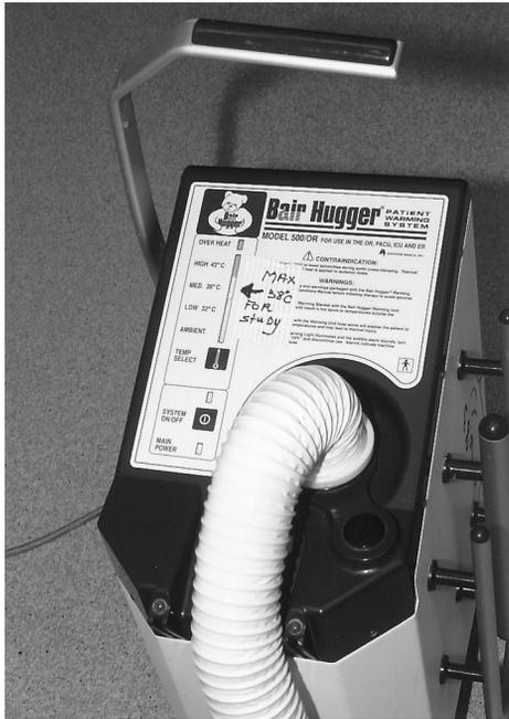
Fig. 1. Experimental forced air warming technique using the hose of a Bair Hugger Model 500 Warming Unit (Augustine Medical, Inc., Eden Prairie, MN). The warming unit clearly identified the medium temperature setting of 38°C.
