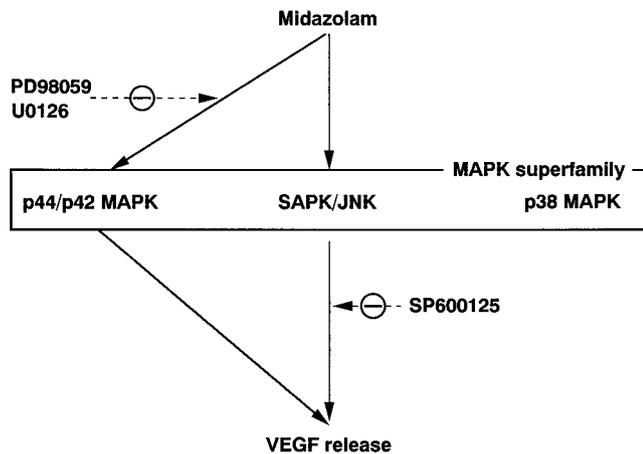
Fig. 10. Diagram of effects of midazolam on VEGF release from vascular smooth muscle cells. Dashed line = inhibitory effect; MAPK = mitogen-activated protein kinase; SAPK/JNK = stress-activated protein kinase/*c-jun* N-terminal kinase; VEGF = vascular endothelial growth factor.
