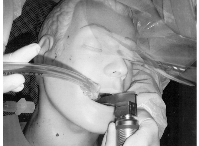
Fig. 1. The bottom edge of the full-face shield is almost pressing on the "patient's" eyes.
