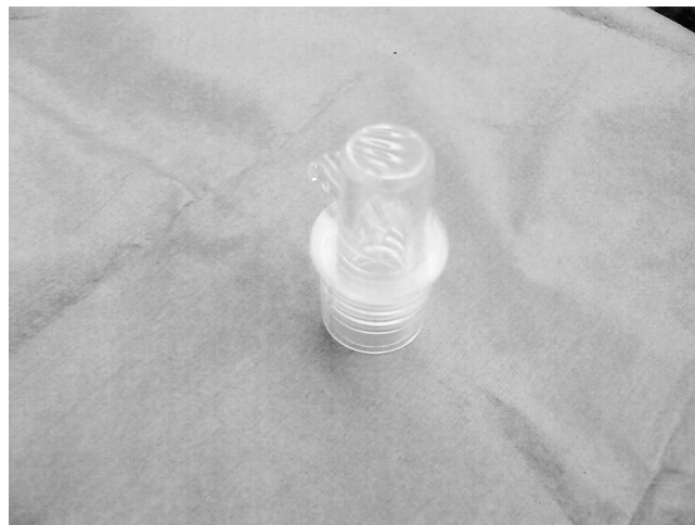
Fig. 1. Straight gas sampling connector (SIMS Portex) with plastic packaging forming an obstructive membrane.
