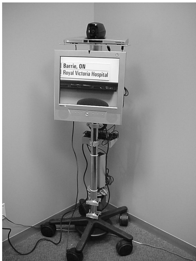
Fig. 1. Portable telemedicine unit with the viewing monitor and camera mounted on the unit.
