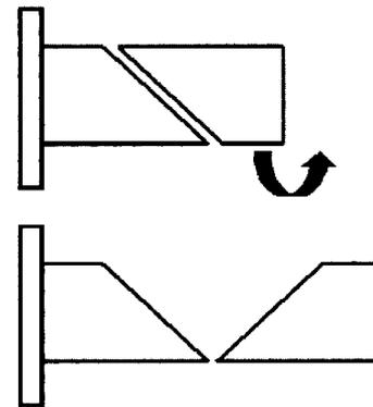
**Fig. 1.** Exaggerated diagrams of the fractured plunger. At top, the fracture is shown reduced, and the shaft is of normal length. Below, the two pieces are rotated into displacement with respect to each other, and the shaft is effectively too long. In our case, the excessive length held the oxygen flush valve partially open at rest.
