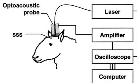
Fig. 1. Optoacoustic system for *in vivo* assessment of changes in oxyhemoglobin saturation in the superior sagittal sinus in sheep.
