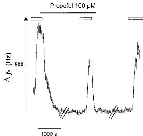
Fig. 3. The effect of 100  $\mu$ M propofol on carotid body chemosensitivity,  $\Delta f_x$  (Hz) at 95%  $N_2/5\%$   $CO_2$  (shaded bars) in one carotid body preparation. Solid line represents perfusion with 100  $\mu$ M propofol for 30 min.
