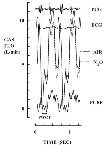
Fig. 1. A whole cycle of pulmonary capillary blood flow (PCBF) tracing (not smoothed), demonstrating the measurement of pulmonary artery pulse wave conduction time (PWCT). ECG = electrocardiogram; N<sub>2</sub>O = nitrous oxide; PCG = phonocardiogram.
