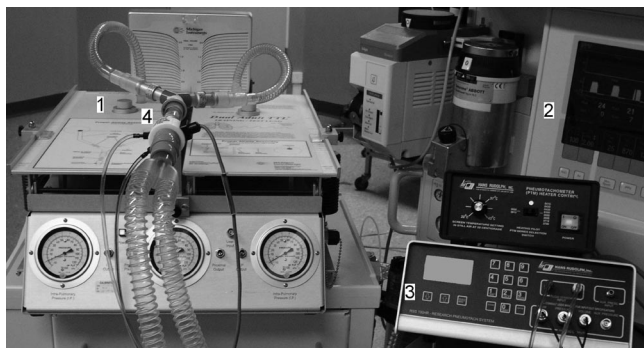
Fig. 1. Setup of the experiment. The two-chamber test lung (1) was connected to the anesthesia machine (2). The pneumotachograph (3) and the pressure transducer were inserted between the endotracheal tube and the Y piece (4) of the respiratory circuit for the continuous recordings of measured flow, tidal volume, and inspiratory pressures.
