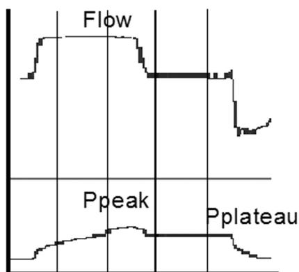
**Fig. 2.** Recorded waveforms of flow and pressure. Total pulmonary resistance was calculated according to the equation: pulmonary resistance ( $R_{plm}$ ) =  $(P_{peak} - P_{plateau})/\text{flow}$ . The use of the laboratory model resulted in no time constant inequalities, and  $P_1$  pressure is not observed.
