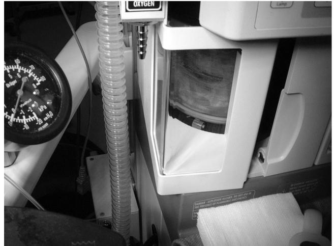
**Fig. 1. Plastic cap under the mechanical ventilator piston.**
