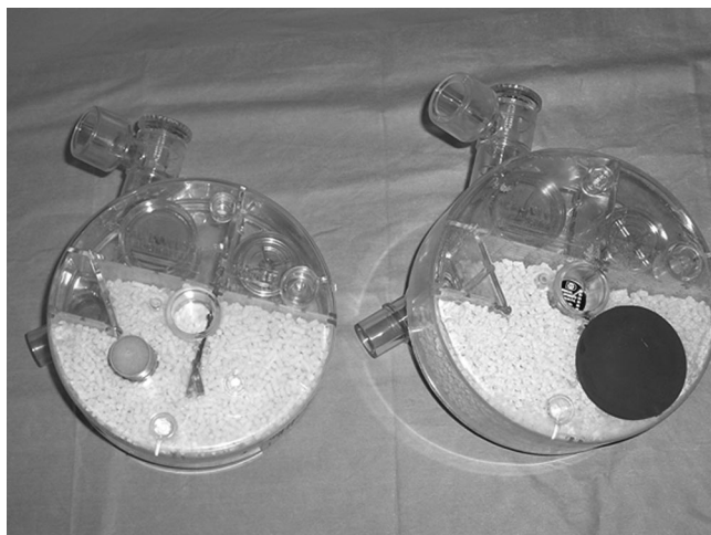
Fig. 2. The disposable absorber with a corked hole made by us on the left side and a reusable absorber with a rubber stopper from the manufacturer on the right side.
