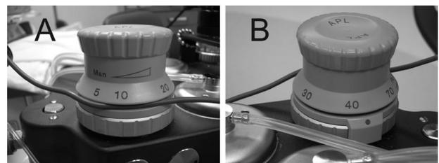
**Fig. 1. (A) Rear view, recreated. Temperature cable trapped between knob and base of the automatic pressure limiting valve. (B) Front view, recreated. Automatic pressure limiting knob shields view of cable trapped beneath knob. Elevation of knob is subtle and easily missed.**
