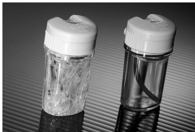
Fig. 2. Water trap that was exposed to isoflurane (left) compared with a normal water trap (right).
