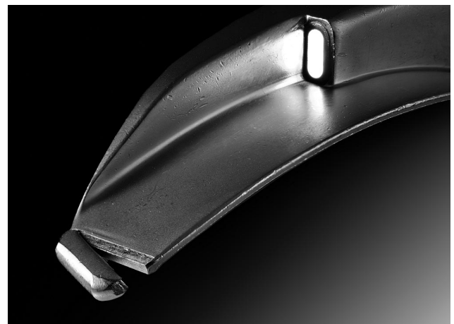
Fig. 1. The loose tip of the laryngoscope blade (partially reattached for illustration purposes) as noticed after cleaning and sterilization.
