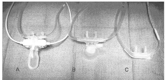
**Fig. 1.** (A) Cap-ONE (Nihon Kohden, Tokyo, Japan), mainstream capnometer system that includes an oral guided nasal cannula. (B) Smart CapnoLine Plus cannula (Oridion Capnography Inc., Needham, MA), a nasal cannula for sidestream Microcap capnometer with oral guide. (C) CapnoLine H cannula (Oridion Capnography Inc., Needham, MA), a conventional nasal cannula (with no oral guide) for sidestream Microcap capnometer.
