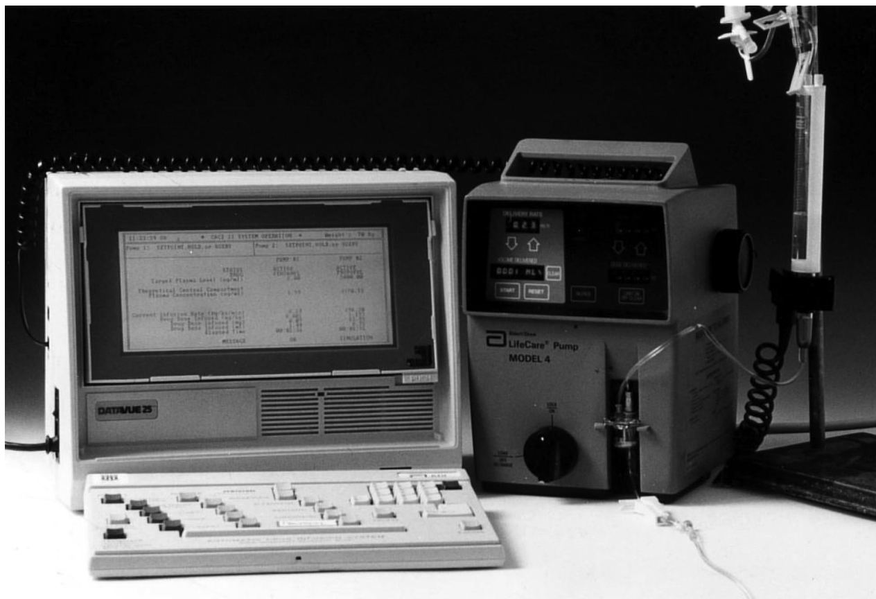
Fig. 1. The present computer-assisted continuous infusion system used at Duke University Medical Center. It consists of a laptop computer electronically linked to an infusion pump. The desired drug plasma or effect-site concentration is entered using the keyboard. Reprinted with permission from Glass PSA, Shafer SL, Jacobs JR, Reves JG: Intravenous drug delivery systems, Anesthesia, 4th edition. Edited by Miller R. New York, Churchill Livingstone Publishers, 1994, pp 389–416.
