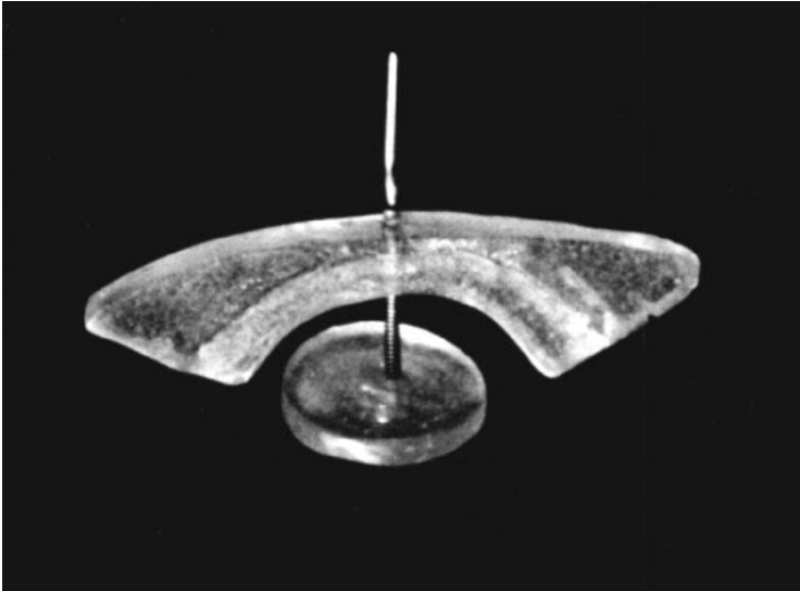
Fig. 1 A lingometer viewed from below, showing the alignment groove that engages the lower anterior teeth. The pin, which is horizontal when in use, is free to move through the acrylic pad that is held by the teeth. The tip of the pin protrudes between the lips, while the inside end is embedded in the button that rests against the tongue.
