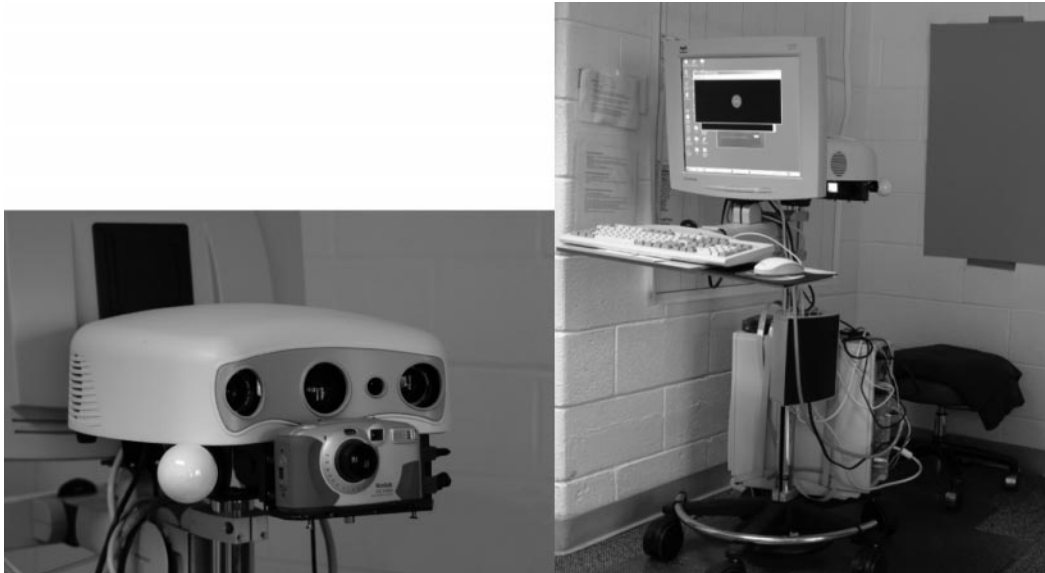
FIGURE 1. The Rainbow 3D camera, Model 250. The system has a central light source with two cameras on each side of the light source and a digital camera in front as shown in the picture on the left. The entire setup with the computer hardware is shown in the picture on the right.
