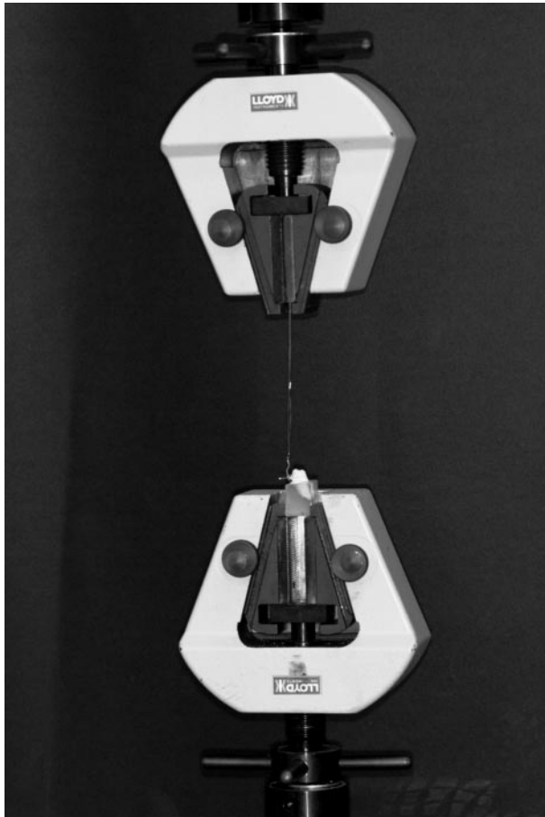
FIGURE 2. Bonded teeth set in acrylic block and positioned in Instron testing machine.
