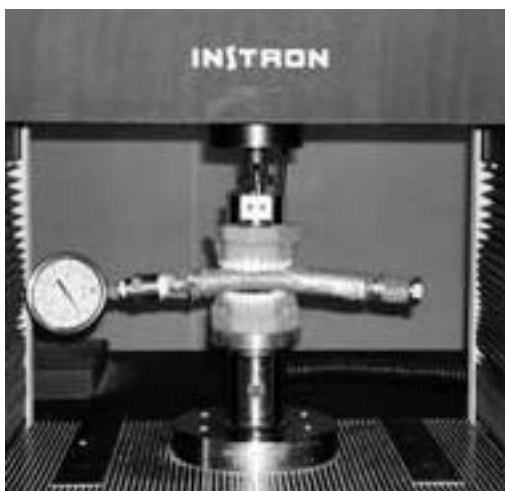
Figure 2. Calibration of the RTBF device in a Materials Testing Machine.
