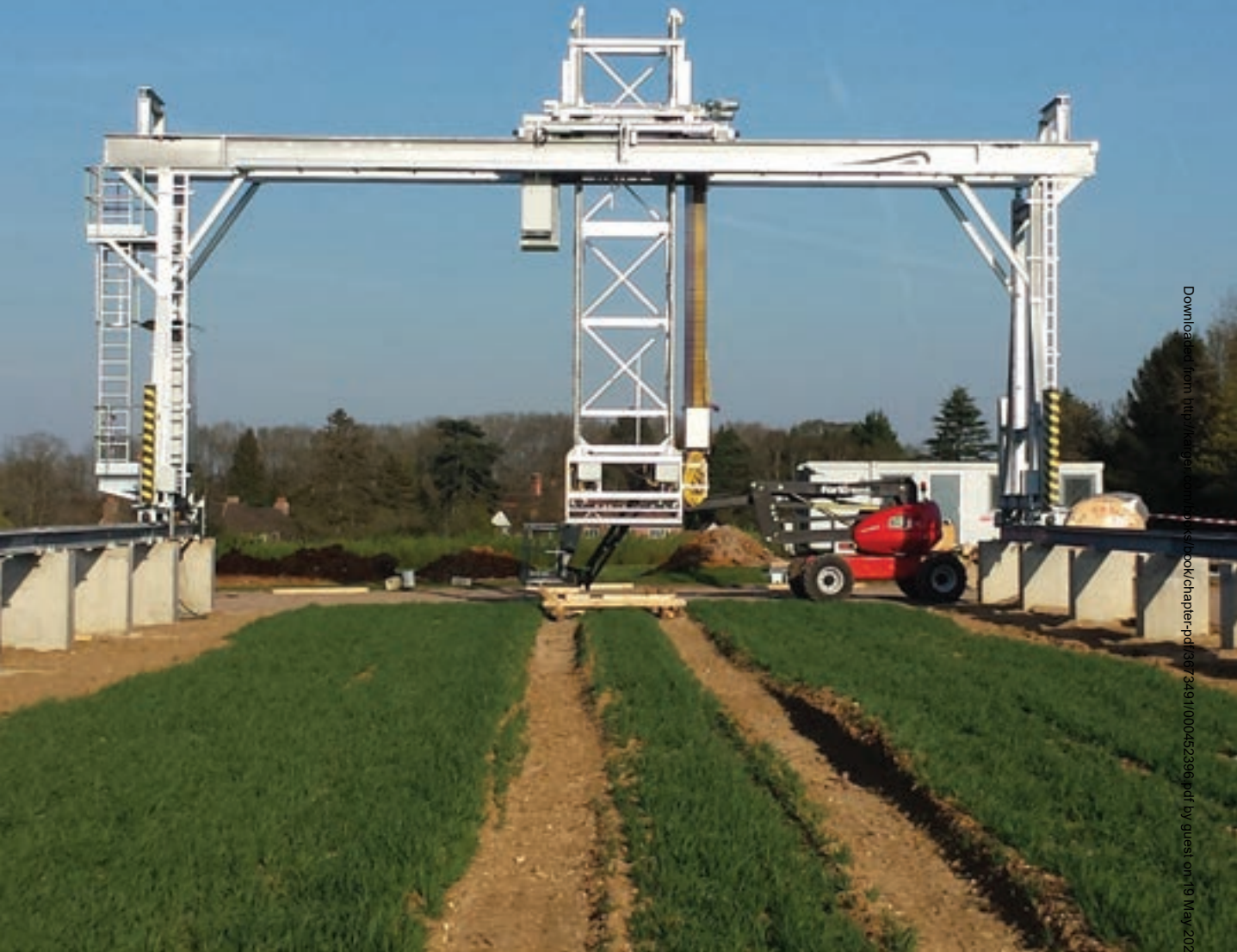
Field scanner at Rothamsted Research – the world's first fully automated field facility for measuring crop growth and health. Source: Achim Dobermann
