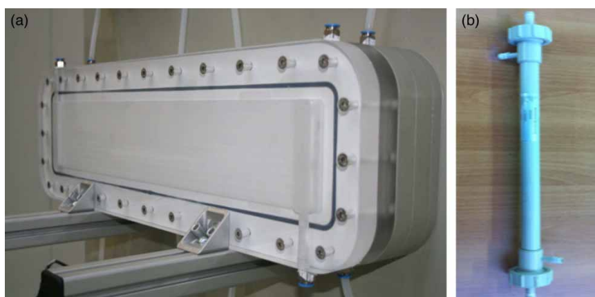
Figure 1 | (a) Aquastill and (b) Microdyn membrane modules used in the study.
