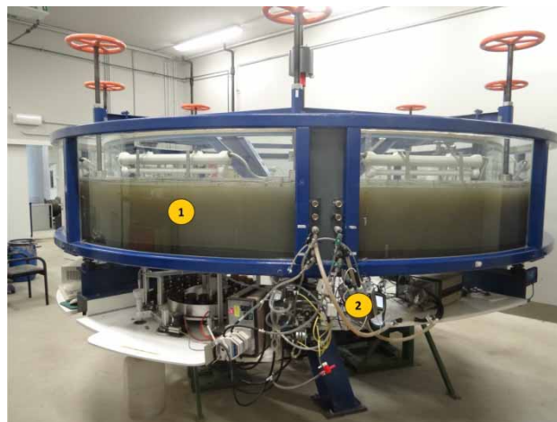
Figure 1 | Annular flume experimental setup: (1) glass channel, (2) measurement unit.
