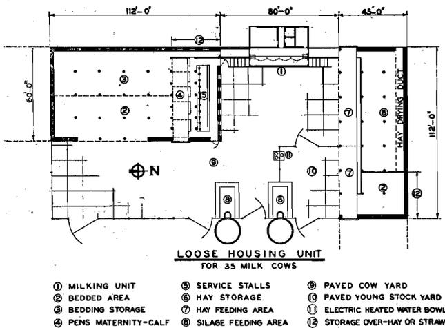
This schematic layout of a 35 cow loose housing system is presented to aid the reader in interpreting the written text. The plan should be expanded to 75 or 100 cows if desired by increasing the length of the resting or bedded area and the hay storage unit.
