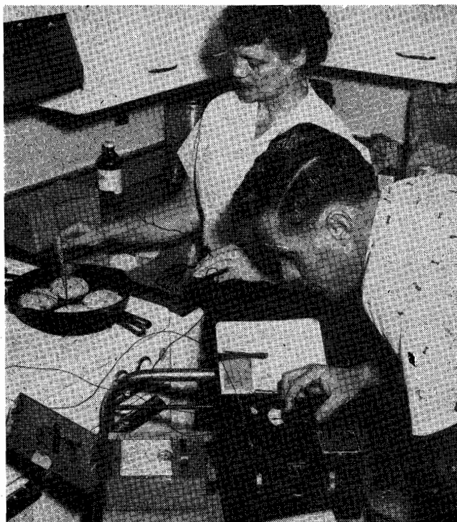
Figure 1. Copper-constantin (24-gauge) thermocouple wires inserted into crab cakes. The terminal ends are connected to a Brown Portable Potentiometer (Model 126 W3).
