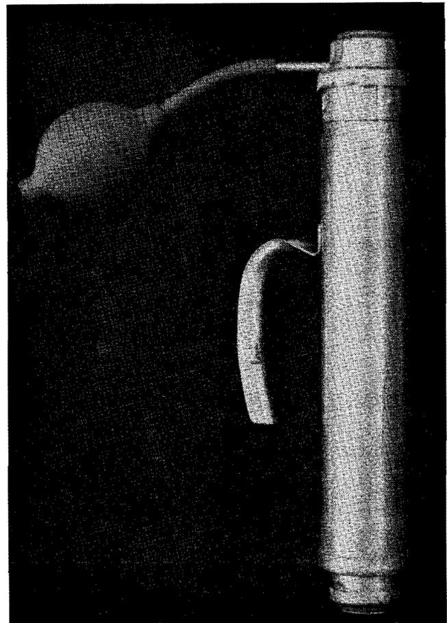
Figure 1. Superior type pressure tester.
