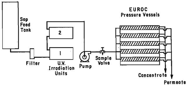
Figure 1. Flow diagram of EUROC maple sap concentration system.
