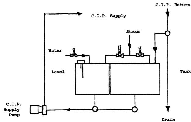
Figure 2. "Re-use" type of CIP system.
