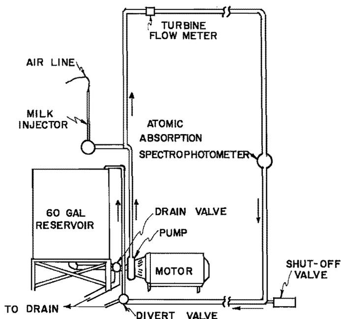
Figure 1. Schematic diagram of the simulated CIP system.
