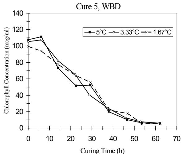
depression tests, three levels of wet-bulb depression (1.67, 3.33, and 5°C, which represent 89, 81, and 70% relative humidity, respectively), were maintained for 64 h at a constant temperature of 35°C. After yellowing (the first 64 h), temperature and wet-bulb depression in the barn were returned to the typical curing schedule values (Figure 1).
