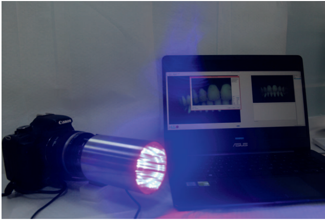
Figure 2. The QLF-D Biluminator 2 camera (Inspektor Research Systems, Amsterdam, The Netherlands) and image-capturing software (C3 v1.20, Inspektor Research Systems).
