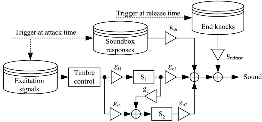
plying coefficients  $g_i$  and  $g_o$ , respectively. In addition, two sample databases are needed for realistic simulation of the soundbox response and the percussive noise caused by key release. In the following, we discuss the string algorithm, model parameters and their control, and the sample databases.
