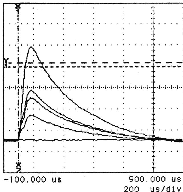
the correct times, in effect a digital audio file of what CSIRAC would have produced at the time if a digital recording device were connected across the loudspeaker terminals. Figure 3 shows an oscilloscope screen image of the reconstructed speaker pulses.
